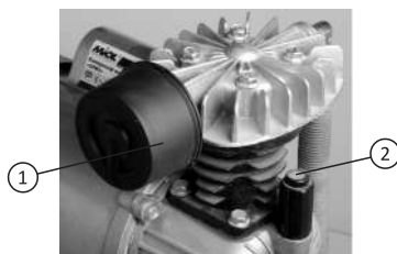
Fig. 3. Installation of air filter 1 — air filter, 2 — drain plug hole
